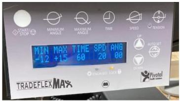
The Auto-Flexion User Interface displays the current Auto-Flexion parameters. The top line displays the parameter name, and the bottom line displays the current parameter.
