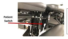
Attach the Patient Switch by inserting the male end of the cable into the Patient Switch Receptacle. The receptacle is on the front end of the table near the left arm rest. NOTE: The Patient Switch must be plugged in for the table to operate.
