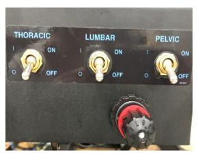
**Auto-Cocking Toggle Switches:** To cock one of the Drops (Thoracic, Lumbar, Pelvic), position the toggle switch to the ON position and depress the Auto-Cocking Control Pedal. To adjust the holding ability (tension) of the drop section, turn the corresponding Drop Tension Control knob to increase or decrease holding ability.
