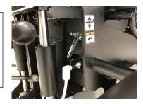
Test the Patient Switch by pressing the button. With the table running, pressing the button once will stop the treatment, a constant audible tone will sound, the table will return to the neutral position and stop. The audible tone can be stopped by pressing the Start/Stop button, which will discontinue the treatment. Pressing and holding the Patient Switch button during the constant audible tone will engage the Comfort Zone.
