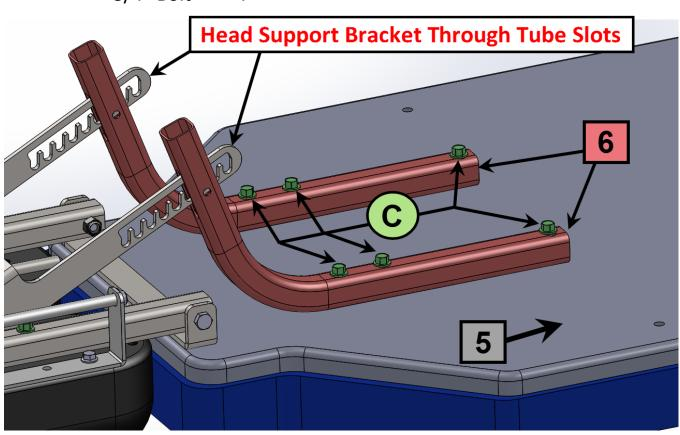
Assembly STEP 5: Attach Head Support Brackets to Head Lock Tubes with
