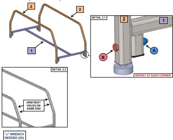
Assembly STEP 2: Attach arm rest to base frame with 2-1/2" Bolt B and Lock Nut .
