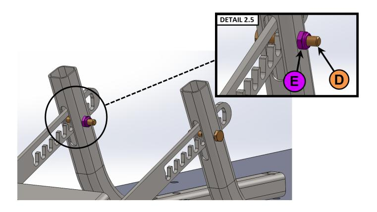
Assembly STEP 6: Attach Top Cushion Assembly to Base Frame with 1-
